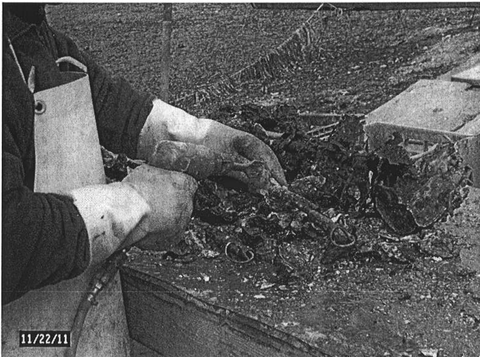
Photo 2. Pneumatic Drill Used to Break Apart Oyster Shell Clusters
