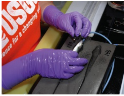
A juvenile salmon is tagged with an electronic sensor and that allows scientists to track its migration.
