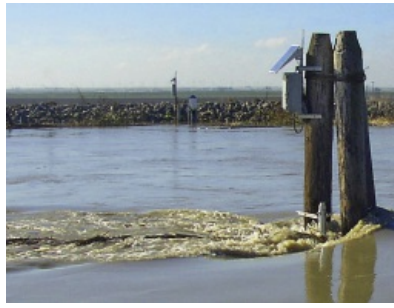
Flow-station instruments mounted on a piling measure direction and amount of water flowing in a Delta channel.
