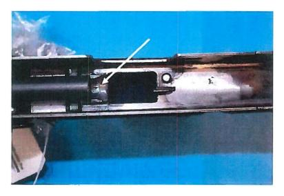
Exhibit 12 lacked a "blocking bar," which is a piece of metal that is welded into the receiver of a semi-automatic firearm to prevent an unmodified machinegun bolt from
